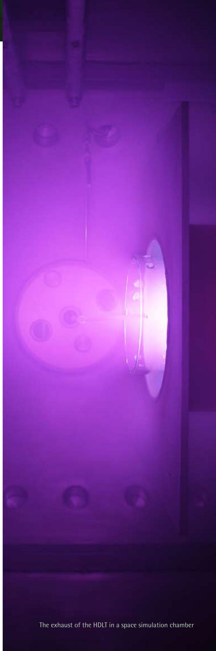
The exhaust of the HDLT in a space simulation chamber
