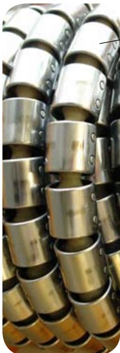
The massive charge at the centre of the accelerator is built up using long rotating chains with links made of alternate insulating and conducting material. These transfer frictional electrostatic charge to the centre of the accelerator tank. The principle is exactly the same as a common Van De Graaff Generator except that in this case, the potential at the accelerator centre reaches 14 million Volts.
