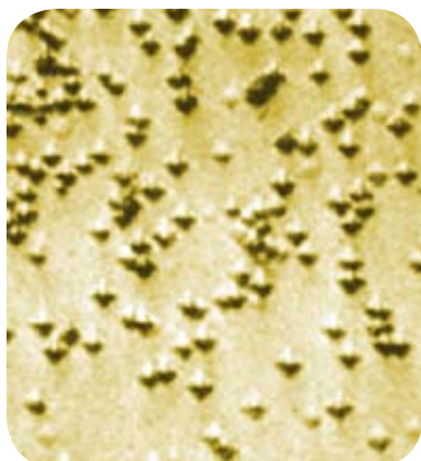
Conical etch pits seeded at high energy ion damage sites
