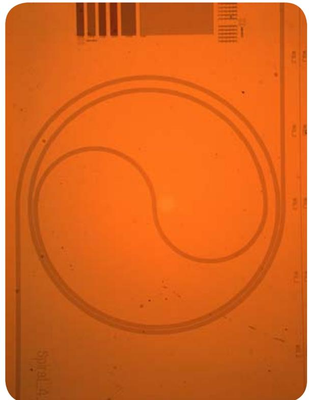
The researchers have produced a chalcogenide waveguide measuring 22cm long, a world record.
