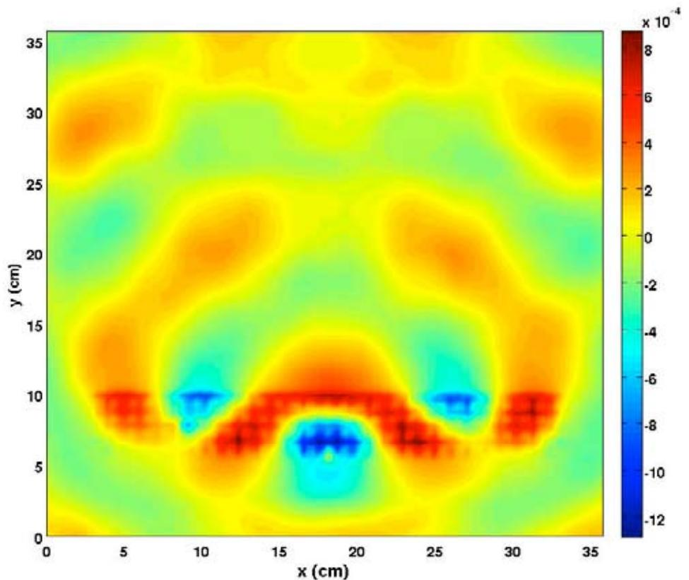
*Laboratory measurement of an electromagnetic wave scattering on a nonlinear metamaterial. The large scale of the microwave based materials enables researchers to more easily measure the spatial behaviour of electromagnetic radiation as it interacts with them.*
