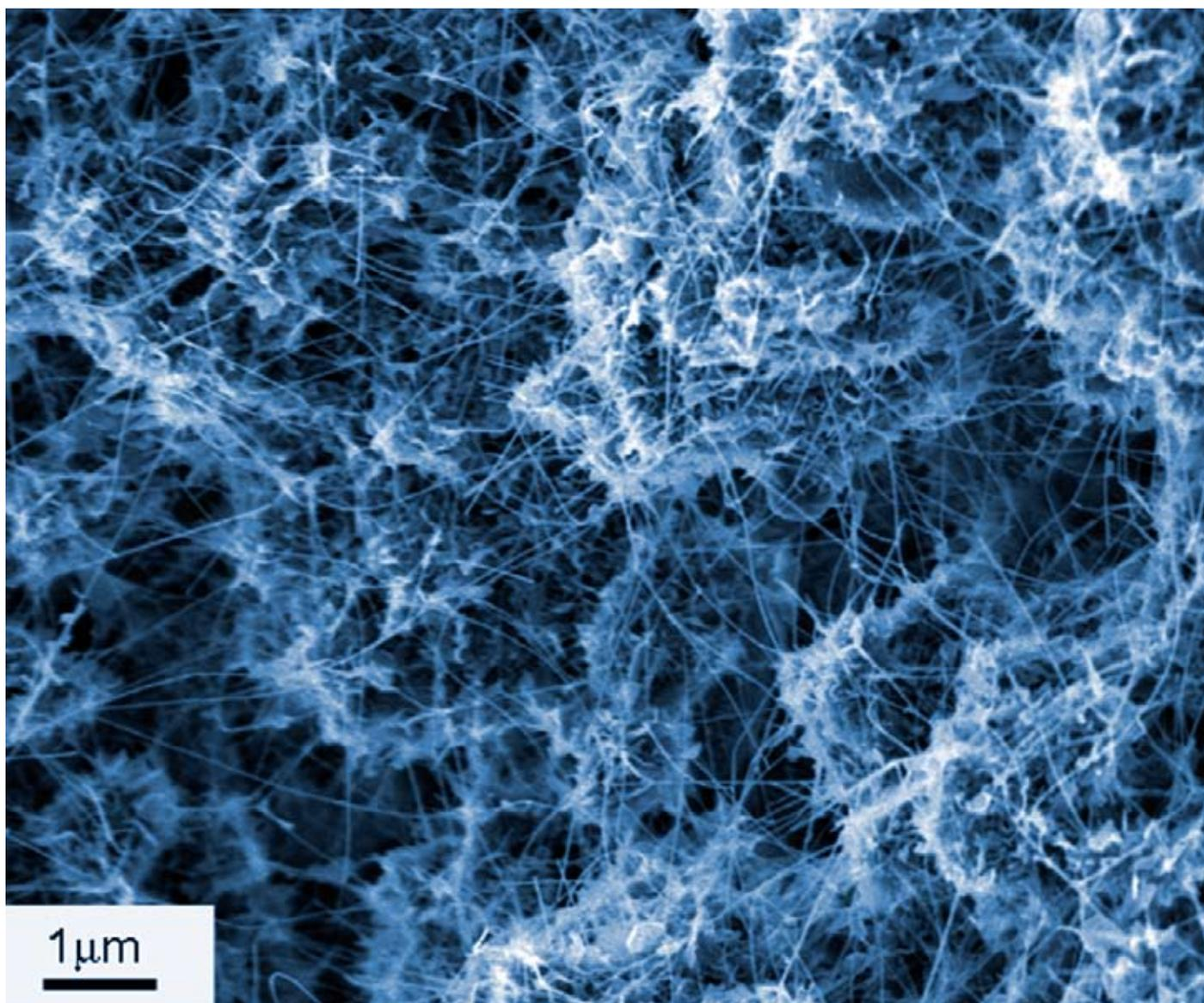
*A scanning electron microscope image of the boron nitride nanotube (enriched with boron 10). They were produced by grinding a powder of the isotope boron 10 in a ball mill for many hours and then heating the crushed powder to around 1100 °C for 6 hours in an atmosphere of ammonia.*
