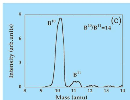
Secondary ion mass spectrometry of a sample of 10BN nanotube sample, showing the dominant presence of 10B over 11B.
