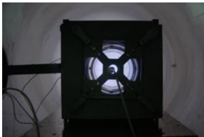
The Helicon Double Layer Thruster in operation inside the space simulation facility at the SP3 laboratory.
