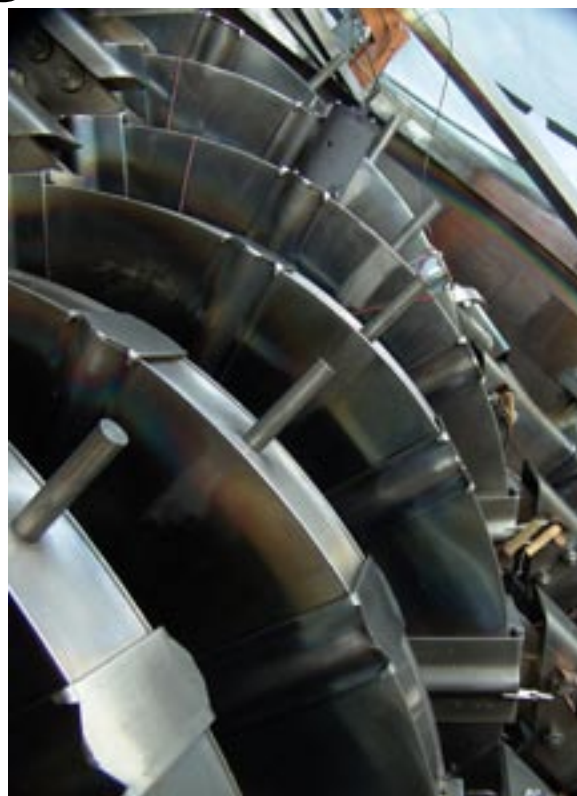
A view along the magnetic confinement coils inside H-1NF. (
