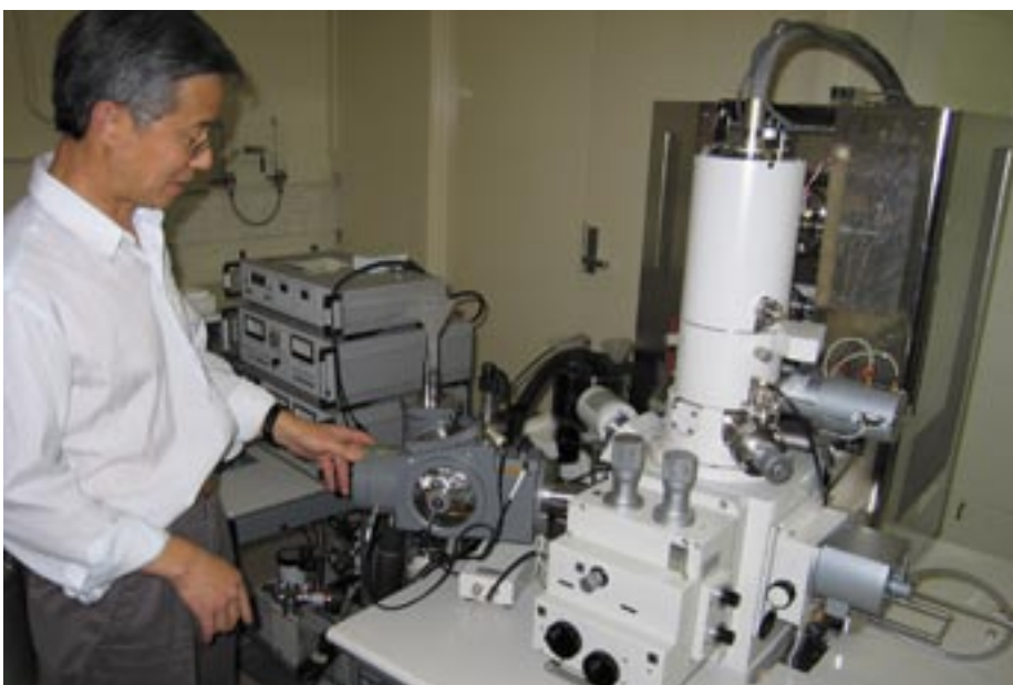
Cheng Huang with the cryo-stage attachment on the Hitachi 4300 Field Emission Scanning Electron Microscope. The cryo-stage makes it possible to work with hydrated and frozen specimens.
