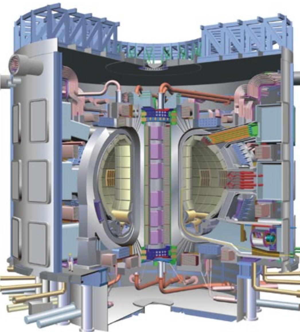
Fusion energy powers the sun and the stars, but it is yet to be tapped by humans. Countries representing over half the world's population plan to construct and operate a large experimental device, ITER (Latin for 'the way'), to demonstrate the feasibility of fusion energy for peaceful purposes. Pictured above is a schematic of ITER experimental device.
