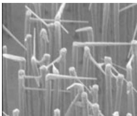
The researchers are devising new ways of growing simple nanowires, compound nanowires and even branched nanowires as shown above. These structures are around 50 nm in width, and they may change the face of optoelectronics.
